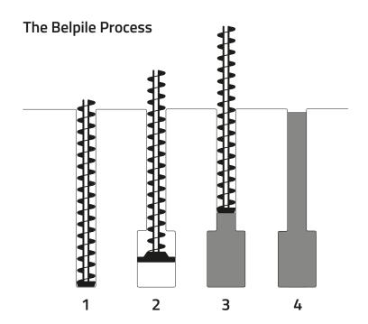
A patented enlarged base piling technique developed and refined by Belpile over the past 30 years
